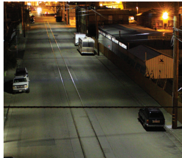
After 40 LED Leotek GreenCobra™ System Power - 47 Watts
