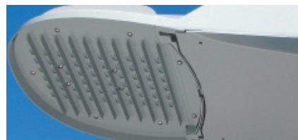
Optional flush-mounted, house-side shield plate can be factory or field installed. The back light strips sharply cut light off at 1/2 mounting height behind luminaire.
